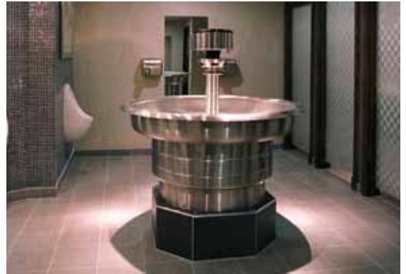
All models utilize less water, energy, and space than lavatories equipped with conventional faucets. A simple, mechanical foot valve or an infrared sensoractivated solenoid valve controls the non-sectional sprayhead.
